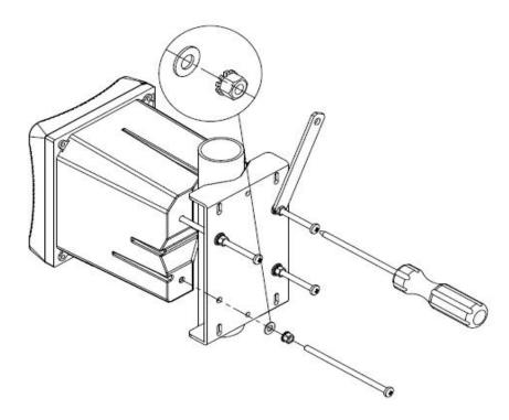
Figure 4 Installation Way of Clamp
