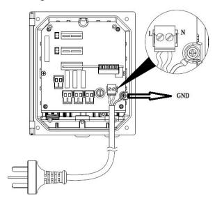
Figure 8 AC220V Power Supply Wiring
