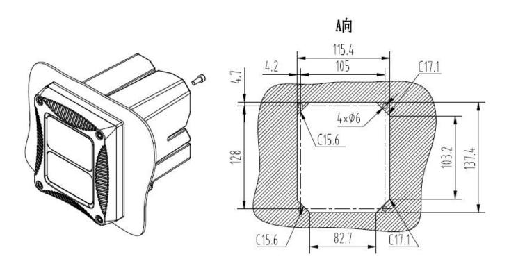
Figure 5 Panel Installation
