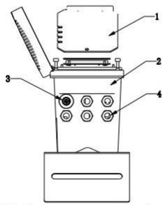
1-High pressure protection board 2-transmitter 3- quick joint
