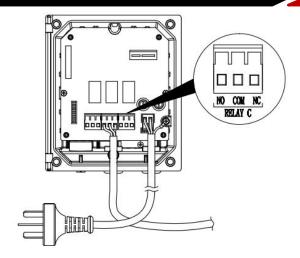
Figure 9 Relay Wiring
