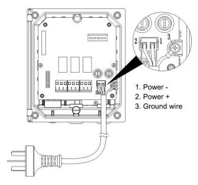
Figure 9 DC 24V Power Supply Wiring
