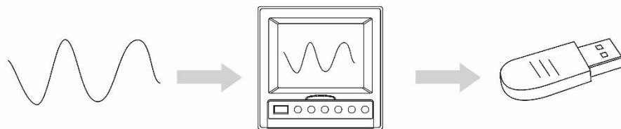
The data that have been saved to an external storage medium can be displayed on a PC using the standard software that comes with the package.
