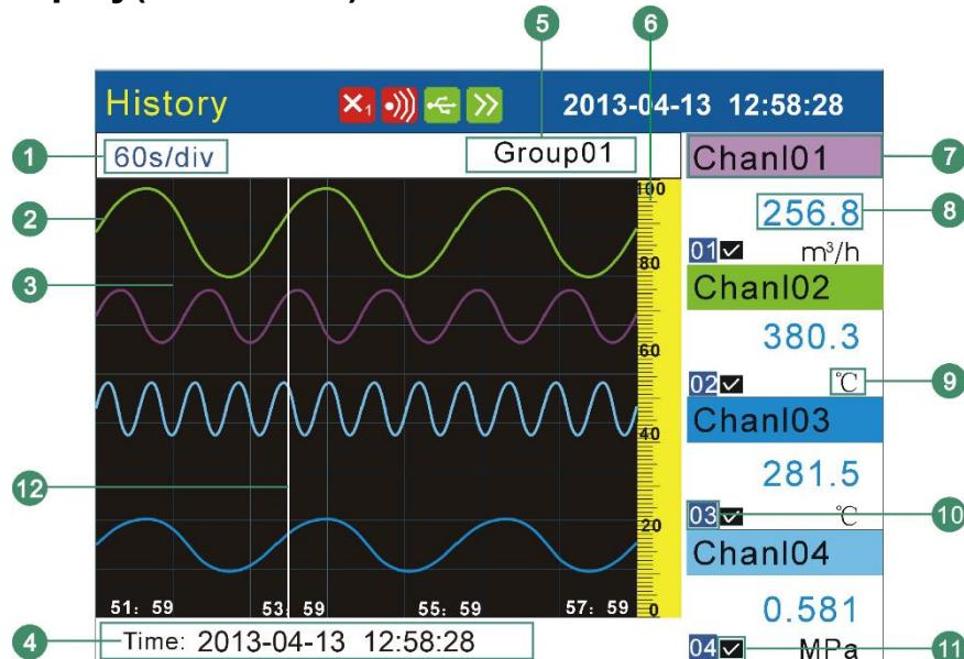
1. Trend cycle. Each grid means the length. The cycle is related with saving interval, Time length = saving interval × Zoom multiple × 30.
