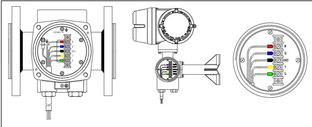
Fig. 5.4.1 Schematic diagram of sensor wiring of remote electromagnetic flowmeter
