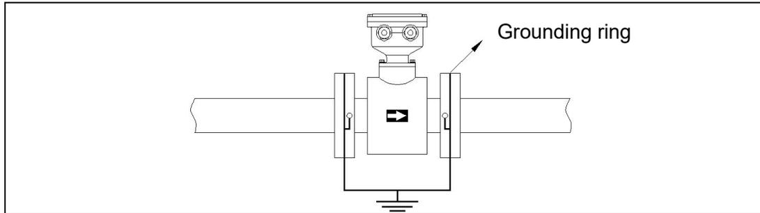
Figure 5.5.3 Installation grounding on insulated pipes.
