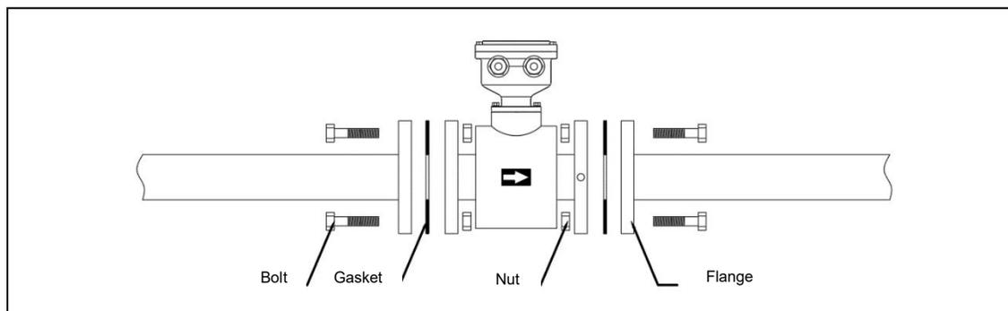
Figure 4.3.2 Installation of remote electromagnetic flowmeter
