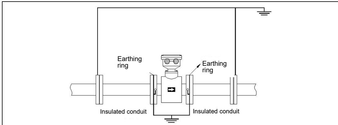
Figure 5.5.4 Grounding in the presence of strong stray current
