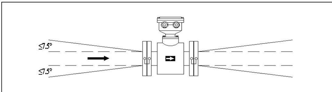
Figure 4.2.2 Installation when the measured inner diameter is inconsistent with the inner diameter of the pipe
