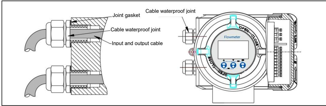
Figure 5.3.1 Schematic diagram of electrical interface.
