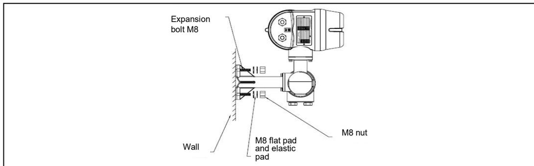
Figure 4.3.4 Install a separation converter on the wall
