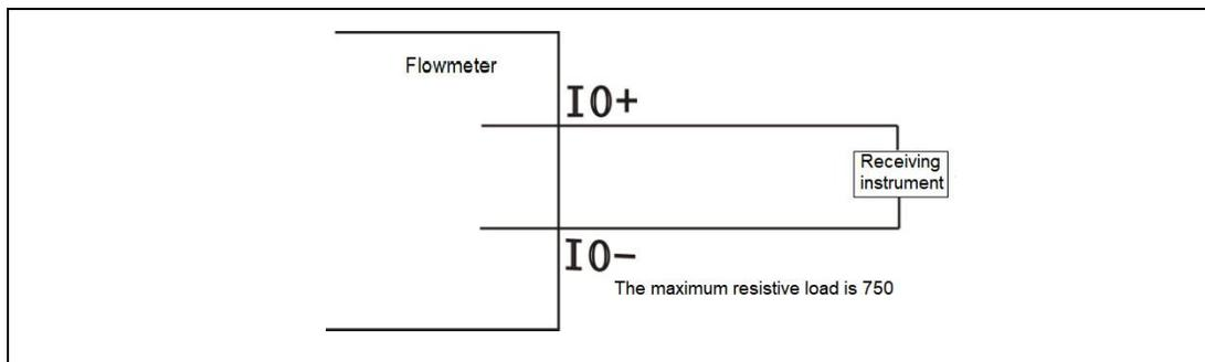
Figure 5.4.4 Current (4~20) mA output connection
