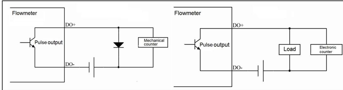
Figure 5.4.5 Passive pulse output connection
