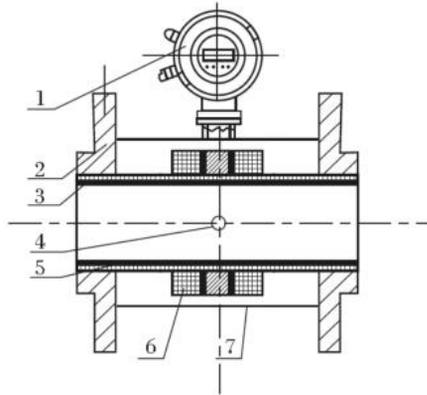
1-converter; 2-flange; 3-insulating lining.
