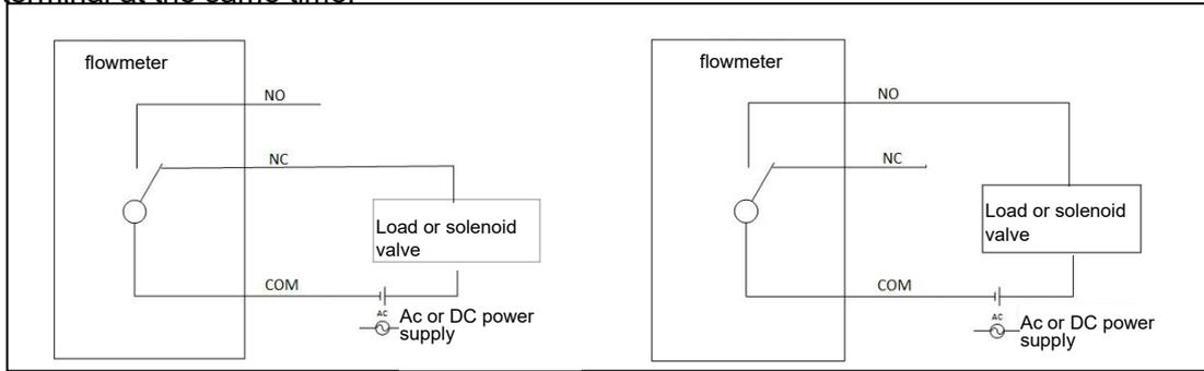
Figure 8.2.1 status output / alarm output connection
