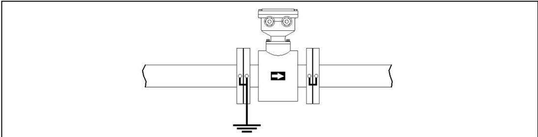
Figure 5.5.2 Installation grounding on metal pipes.
