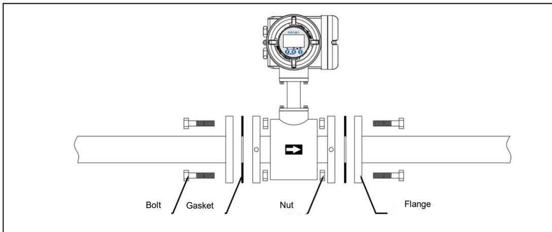
Figure 4.3.1 Installation of integrated electromagnetic flowmeter
