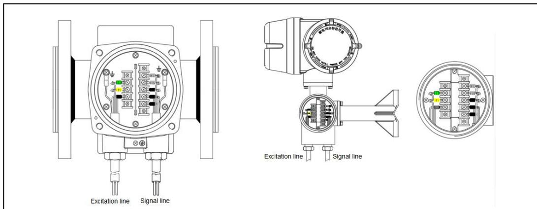
Fig. 5.4.2 Wiring diagram of remote electromagnetic flowmeter sensor
