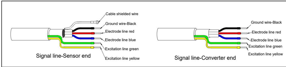
Figure 5.2.1 Schematic diagram of standard cable
