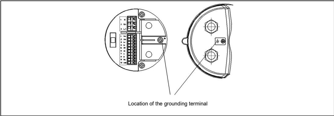
Figure 5.5.1 Converter grounding
