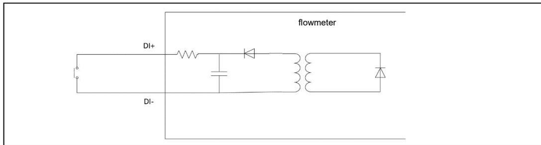
Figure 8.2.2 status input connection
