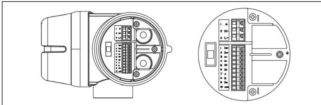
Figure 5.3.2 Schematic diagram of input and output terminals
