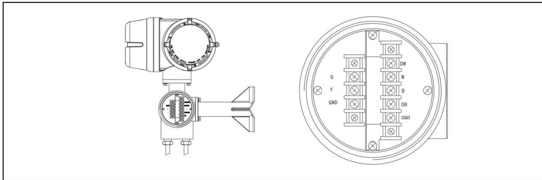
Figure 5.3.6 Schematic diagram of the terminal of the separation converter
