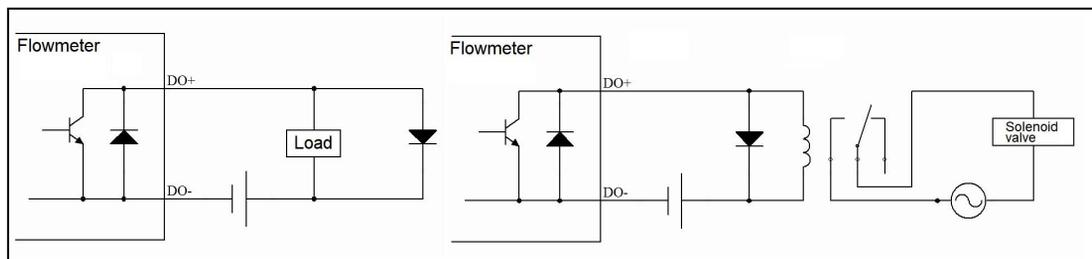
Figure 5.4.7 Status output / alarm output connection
