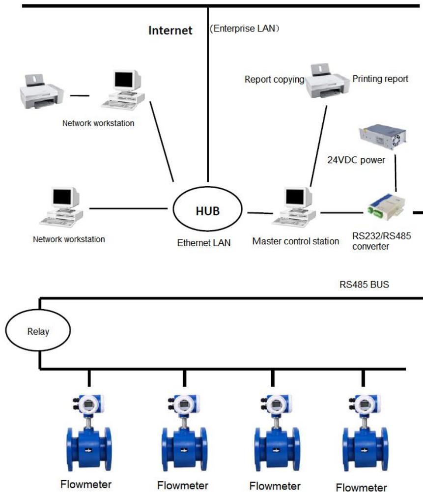
Figure 9.1.1 typical network connection
