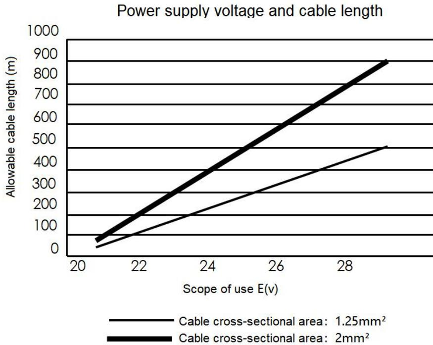
Figure 5.4.3 DC power supply voltage and cable length
