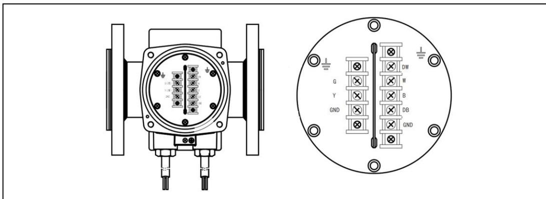
Figure 5.3.4 Schematic diagram of the terminal of the separation sensor
