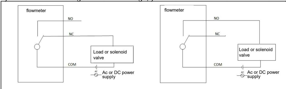
Figure 5.4.9 Relay output connection (left-normally closed, right-normally open)
