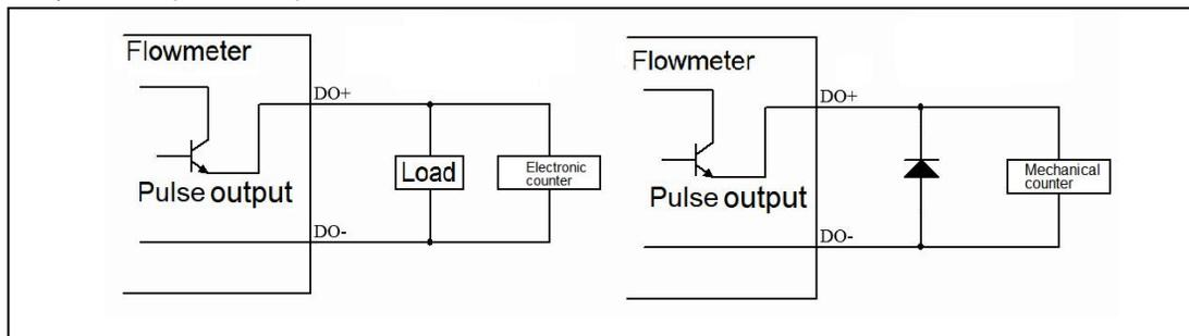
Figure 5.4.6 Active pulse output connection
