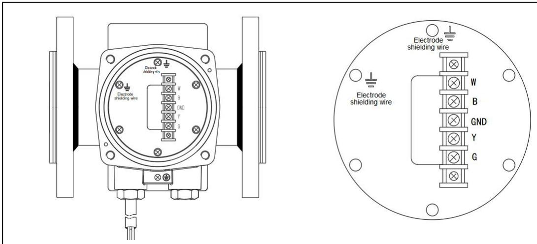
Figure 5.3.3 Schematic diagram of the terminal of the separation sensor (standard cable A)
