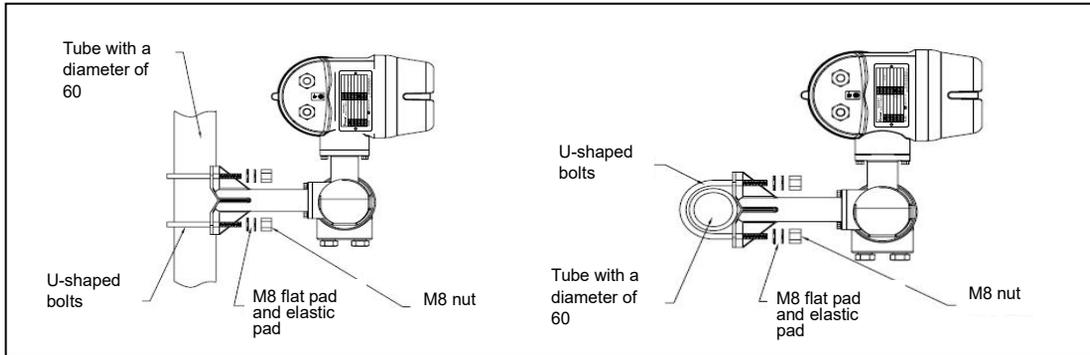
Figure4.3.3 Install a separation converter on a steel pipe
