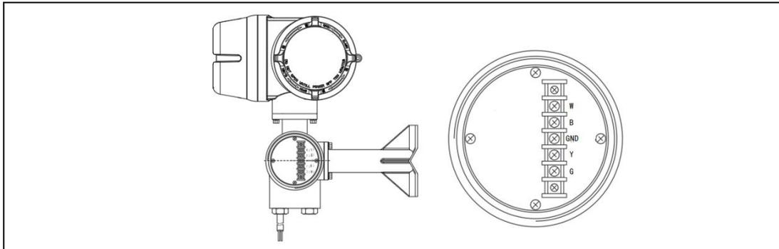
Figure 5.3.5 Schematic diagram of the terminal of the separation converter (standard cable A)
