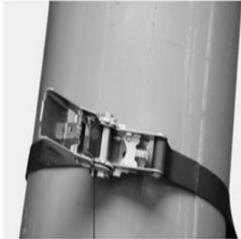
Pass the tape through the transverse groove in the middle of the tensioner's rotating shaft and tighten it by hand.
