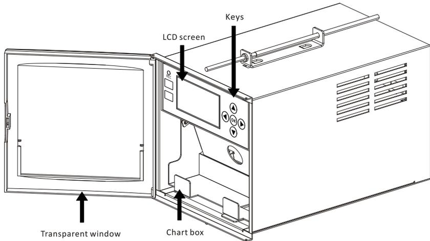
Transparent window; LCD screen; chart box; keys; chart box bottom
