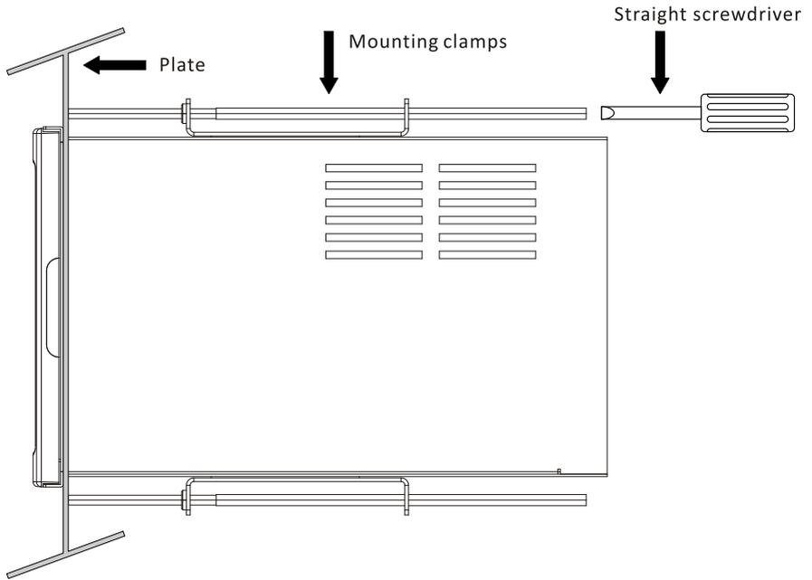
Insert the recorder from the front of steel plate of 2-12 thickness and install mounting clamps and use the straight screwdriver to tighten under an appropriate strength. Make sure that the recorder is horizontal.
