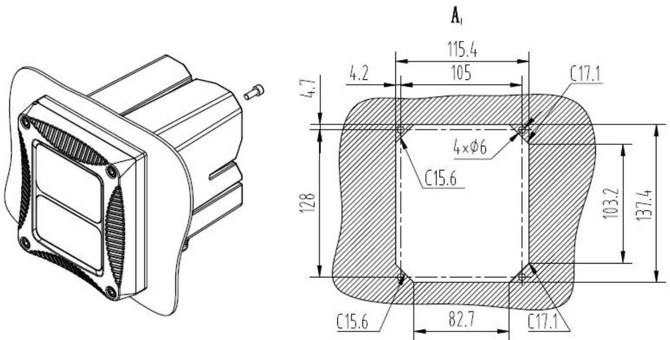
**Figure 5 Panel Installation**
