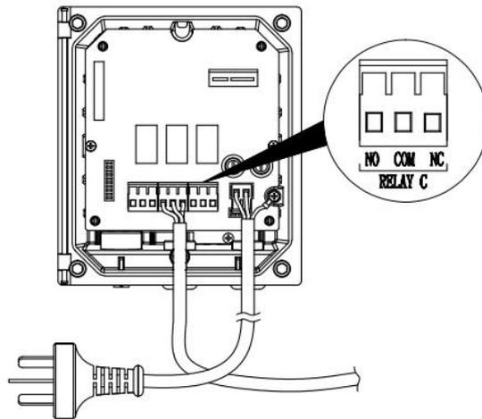
**Figure 9 Relay Wiring**
