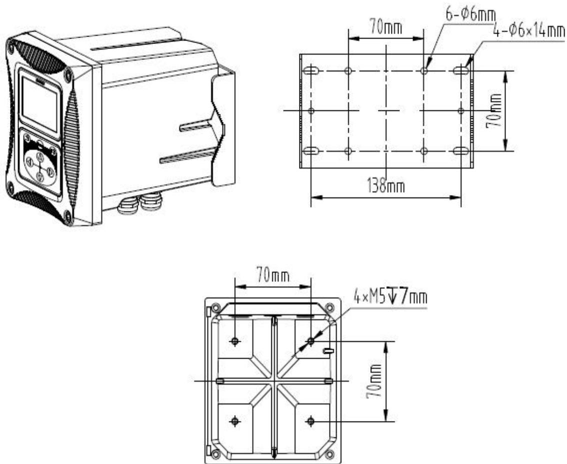
**Figure 3 Installation Size**
