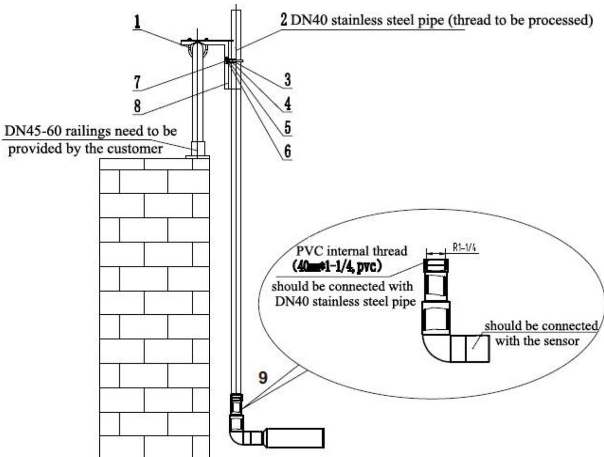
Figure 11 Schematic Diagram on the Installation of Sensor
