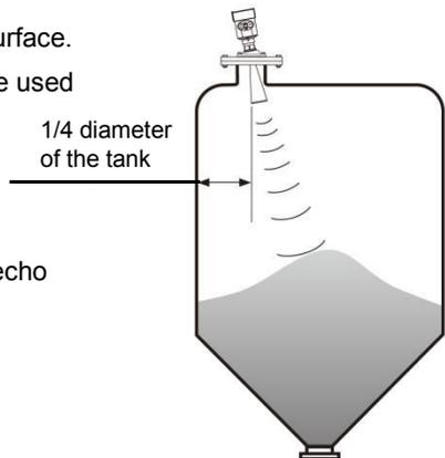
(Due to the solid surface tilt will cause the echo attenuation, even loss of signal.)
