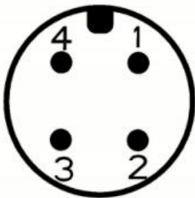
Fig.15 Diagram of aviation connector (M12×1)
