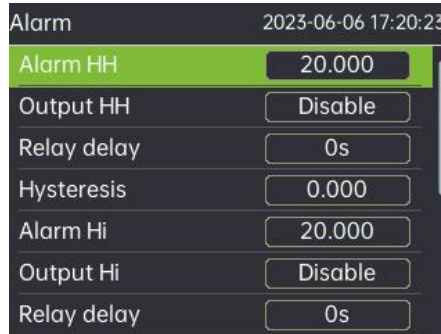
Figure 12 Alarm setting interface
