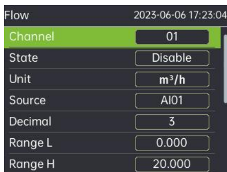
Figure 18 Flow setting interface
