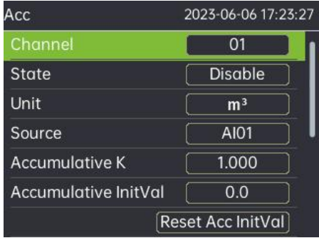
Figure 19 Accumulation setting interface
