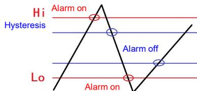
Fig.18 High- or low-level alarm and Hysteresis
