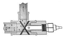
Right: part of the fluid in the pipeline flows through the conductivity cell and is constantly updated, so the measurement is accurate, and the opening of the sensor must face FLOW.
