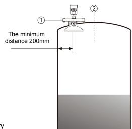
The top conical tank level, can be installed at the top of the tank is intermediate, can guarantee the measurement to the conical bottom.
