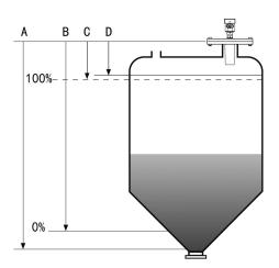
**Datum measurement:** Screw thread bottom or the sealing surface of the flange.
