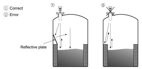
The role of the reflecting plate is refracted away the obstacle signal.
