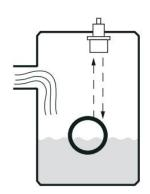
The transducer should not be mounted too close to the tank wall, the bracket can cause strong false echoes.
