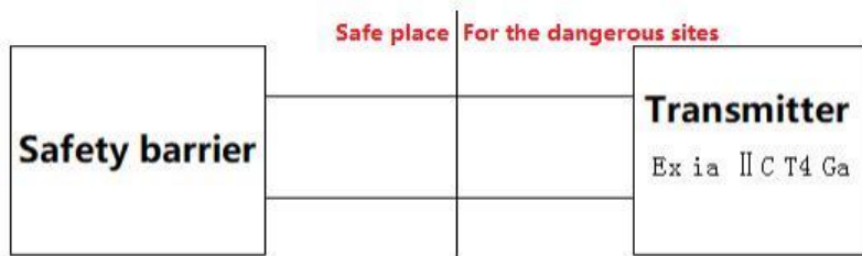
The connection diagram of the power cord of the explosion-proof transmitter
